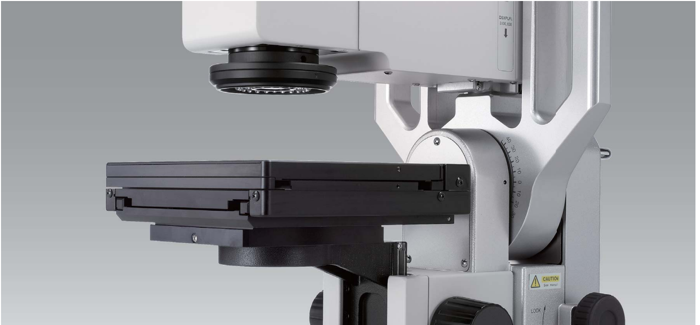
Motorized stage with 100 mm x 100 mm stroke
