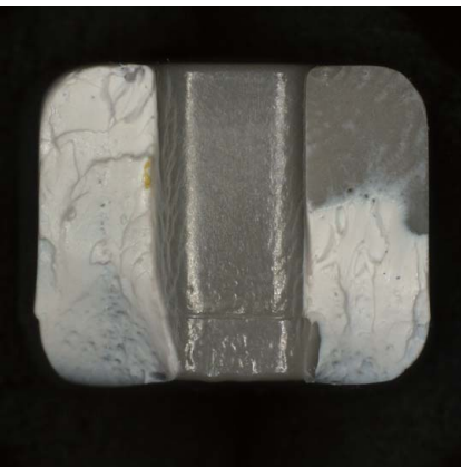
Fractured resin surface
